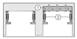
If the installation niche is deeper than the appliance, a solid wooden beam (1) can be placed behind the anti-tip brackets (2) so the appliance can be securely attached to the base or wall.
